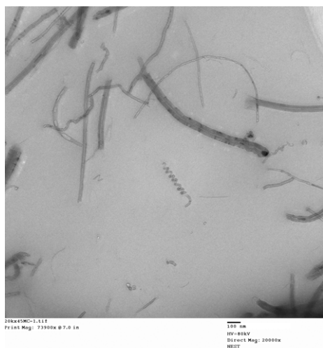
Figure 2. TEM image of the MWNTs/PVA nanofibres treated by methanol/crosslinking.
